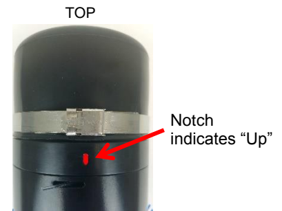
FIGURE 3-6 Hydrophone Mounting Orientation
